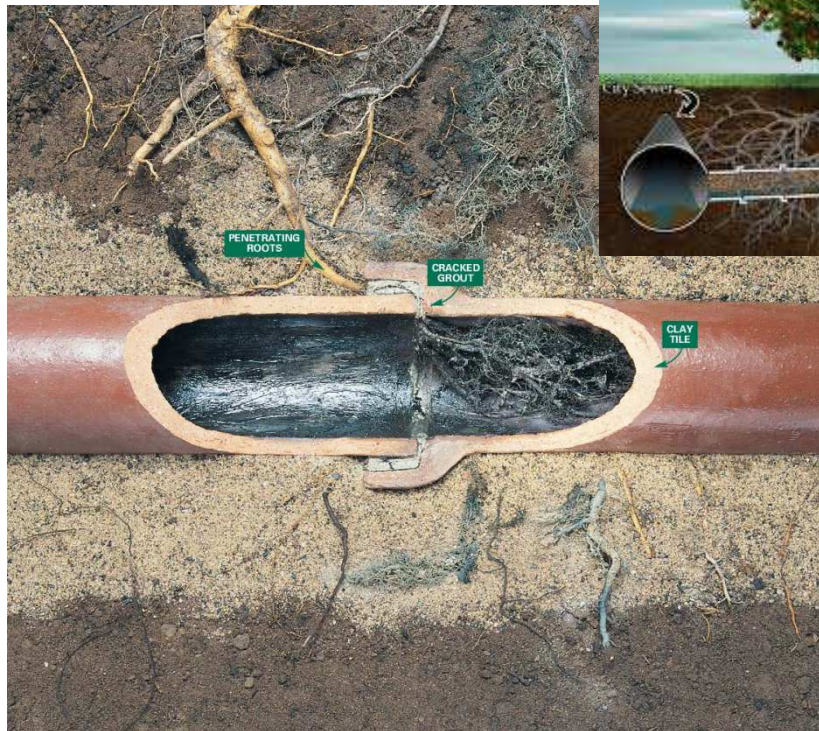
Typical Examples Sanitary Sewer System Tree Root Damage
