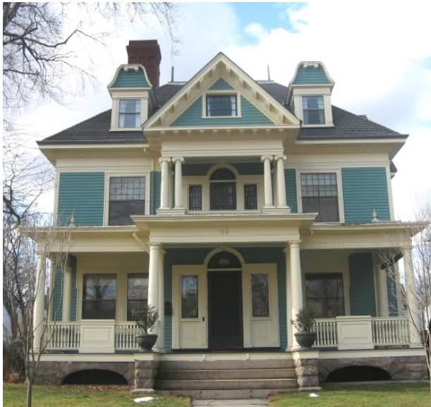
The house at 69 Lexington Street is an elaborate example of an Colonial Revival house, with its symmetry, hipped roof, dormers, sidelights and fanlight, double-hung windows, and porch.
